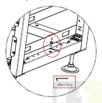
Twist one end of the cable harness (8) in 4.8 to the wiring position shown in the figure, and twist the other end to the ground copper bar of the PDC using an Allen wrench.
