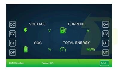
**6** After the setting is successful, you need to restart. Click the Start button to restart, wait for about 8 seconds until the yellow HV light indicator comes on.
